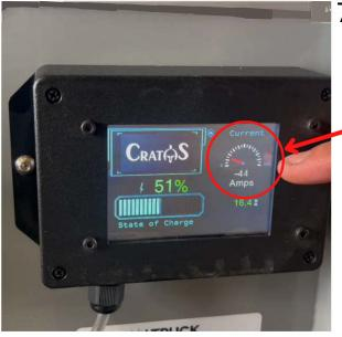
7 - Wait 30 seconds, the meter should read at (or close to) -44 amps.
